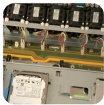
Horizontal 6Gb/s SATA backplane with smart fan control
