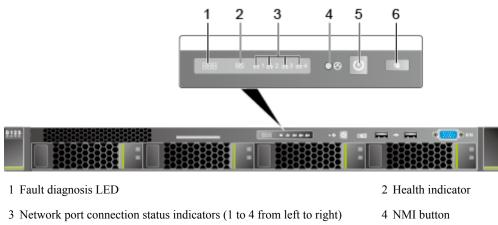
• Figure 4-11 shows the indicators and buttons on the front panel of a server with eight 2.5-inch hard disks.
