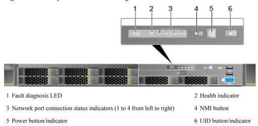
• Figure 4-12 shows the indicators and buttons on the front panel of a server with ten 2.5-inch hard disks.
