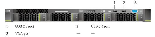
• Figure 4-7 shows the ports on the front panel of a server with eight 2.5-inch hard disks.
