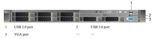
• Figure 4-8 shows the ports on the front panel of a server with ten 2.5-inch hard disks.
