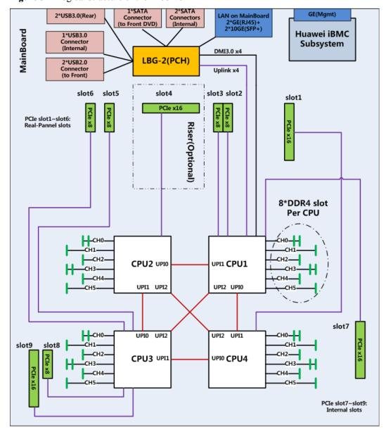
Figure 3-1 Logical structure of the 2488 V5
