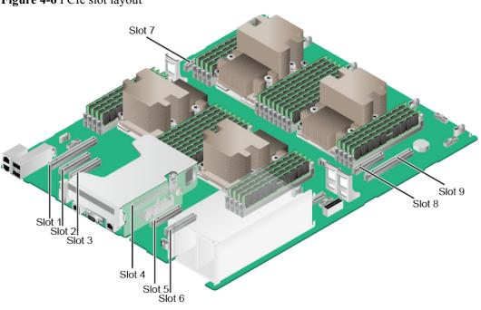
Figure 4-6 PCIe slot layout
