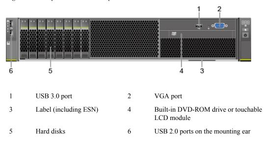
Figure 4-2 shows the components on the front panel with 25 SAS/SATA hard disks.
