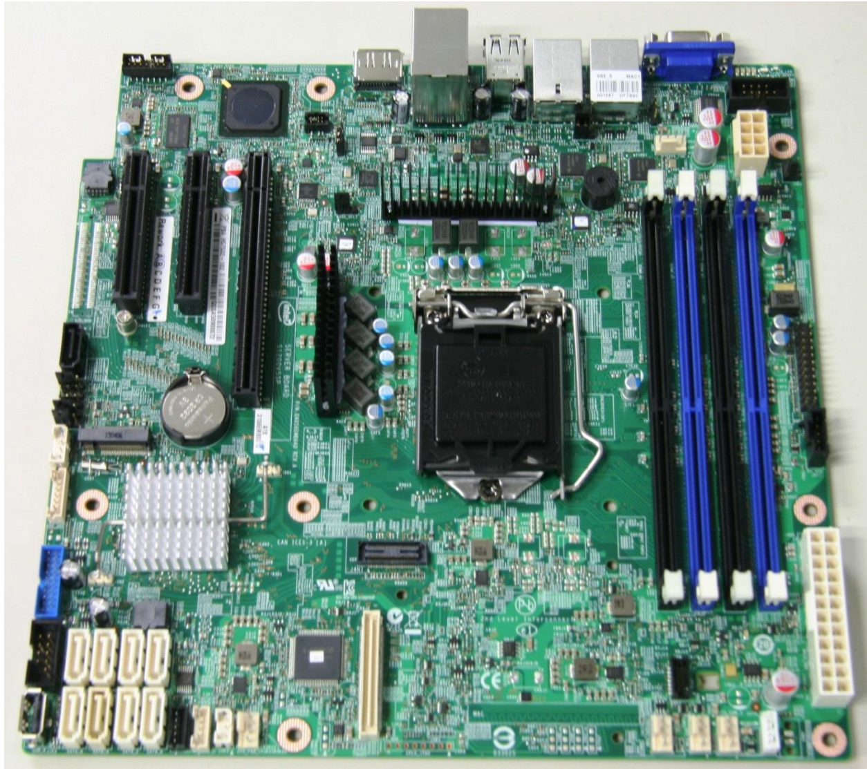
Figure 1. Intel® Server Board S1200SP Layout (S1200SPL)
